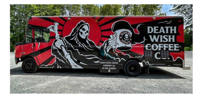
The DOL Max overlaminate provides excellent durability of up to 7 years vertical and up to 2 years horizontal.
