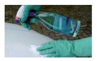
**5.** Treat the surface with Avery Dennison Surface Cleaner prior to any new application of self adhesive film.
