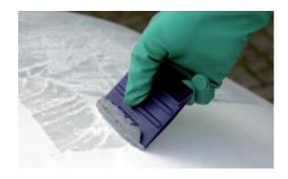
**4.** Use a squeegee to remove the glue from the surface. Be careful to avoid scratching. This procedure can be repeated if necessary.
