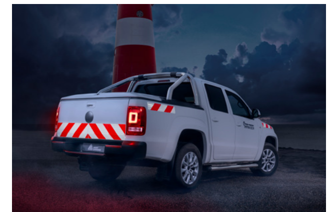
Avery Dennison Chevron White/Red used for vehicle marking according to DIN30710 and TPESC-B.
